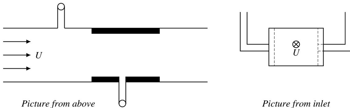
Consider steady water flow filling a rectangular pipe with constant height. The width of the pipe is mostly constant, but in one region the inner of the pipe is narrowed to 80% of the width. The water velocity in the wide region is 1 m/s.
