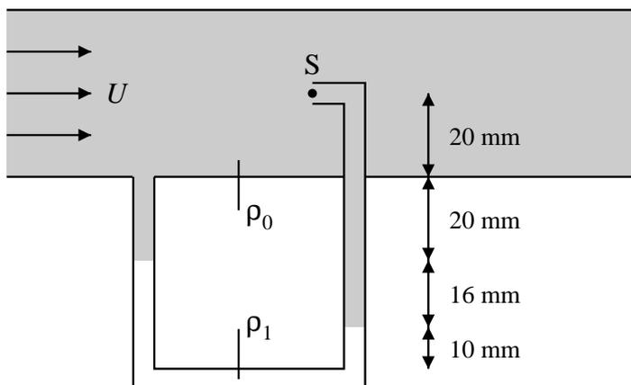
The figure above illustrates a steady water flow in a pipe. A small tube is connected at the bottom of the pipe, and returns into the pipe as a Pitot tube. The Pitot tube is directed towards the flow and the point  $S$  at the entrance is a stagnation point where the fluid velocity is 0. The lower part of the by-pass is filled with mercury, while the rest is filled
