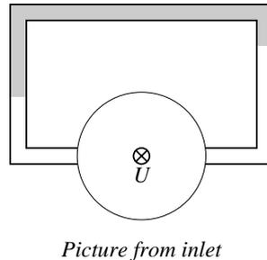
The brilliant(?) idea is to attach a small tube as shown in the figure. The tube is in part filled with water with density  $\rho_0$ , and in part (the upper, grey region in the figure) with a fluid with density  $\rho_1 < \rho_0$ .
