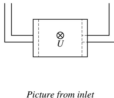
Consider steady water flow filling a rectangular pipe with constant height. The width of the pipe is mostly constant, but in one region the inner of the pipe is narrowed to 80% of the width. The water velocity in the wide region is 1 m/s.
