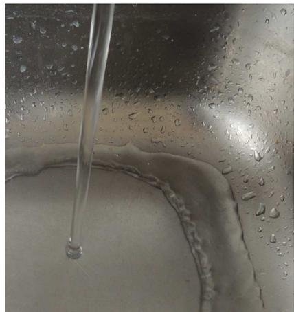
Look at the bottom of the sink. There is a sudden change from thin, radial flow to much thicker, less orderly flow. Watching the flow in real life shows that the “edge” is stationary. Can we understand it?
